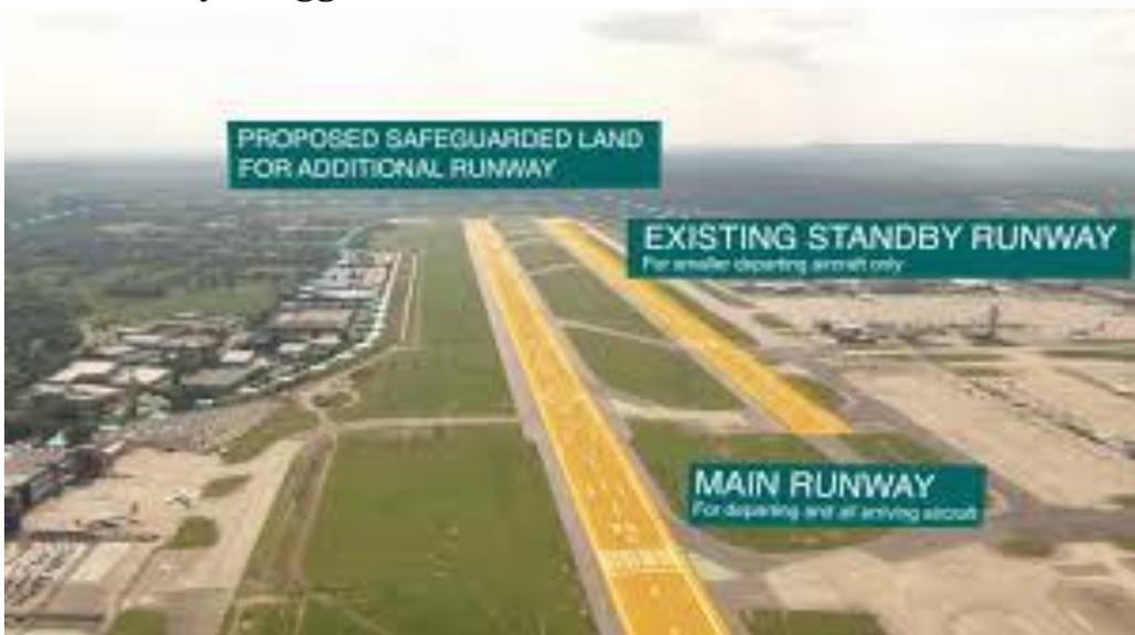
*Gatwick’s current plans are to move the standby runway a few yards to the north (to the right in this diagram) and use it at the same time as the main runway. And to build a second main runway (to the far left in this diagram).*
